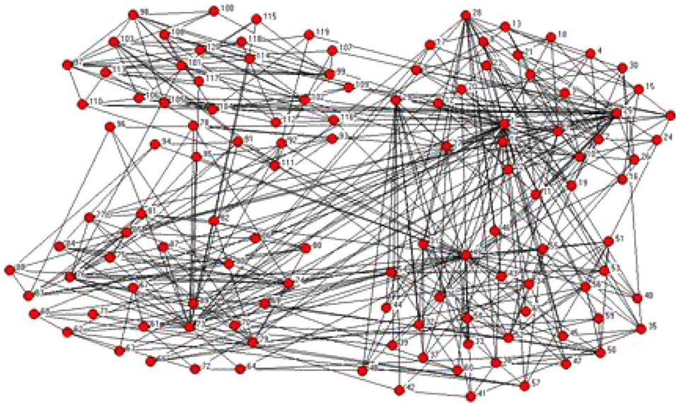
FIG. 2. (Color online) A simple scale-free network with communities generated by our model. In this case there are four communities, N=120 , m_0=m=4 , n=1 , and c=4 .
